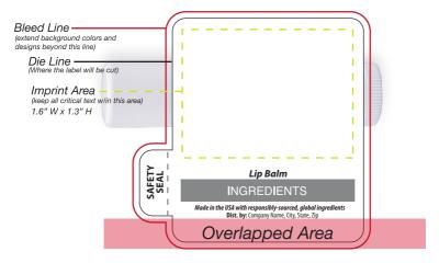
Do not place anything in the Overlapped Area as this will be covered up when the label is wrapped around the lip balm tube.
