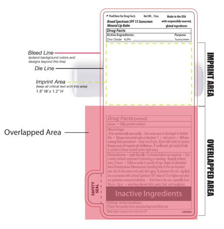
Do not place anything in the Overlapped Area as this will be covered up when the label is wrapped around the lip balm tube.
